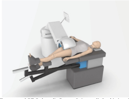
The proposed QT Orthopedic Scanner being applied to hip imaging Image 11
