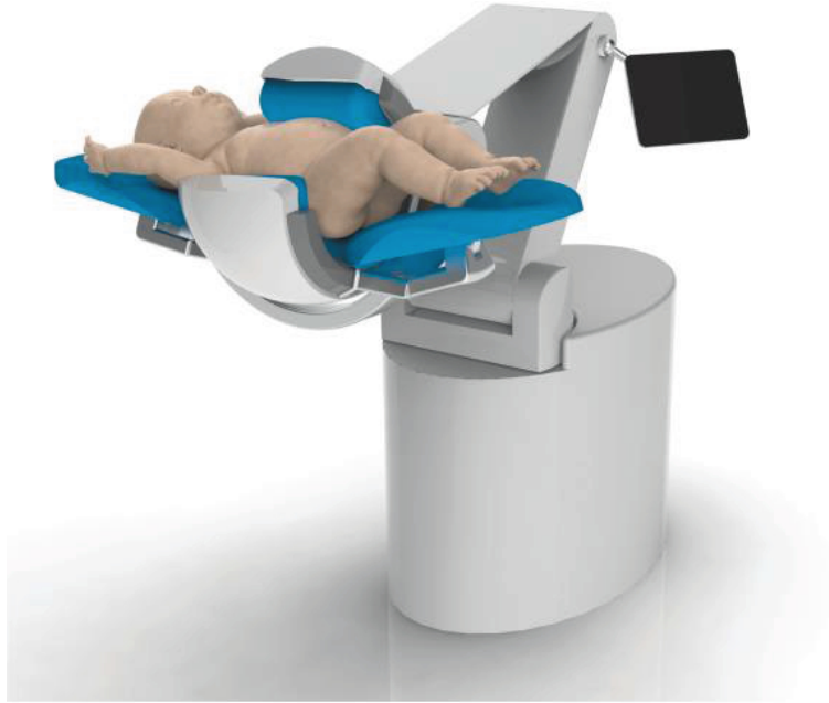
The Open Partial Angle Scanner will be applied to infant body imaging in the proposed QT Infant Scanner (concept drawing)
