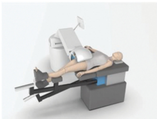
The proposed QT Orthopedic Scanner being applied to hip imaging
