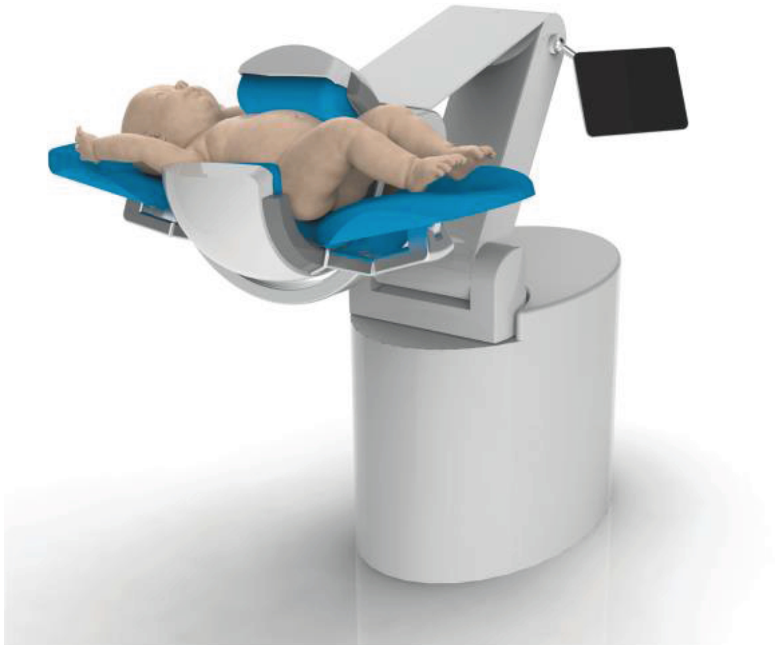
The Open Partial Angle Scanner will be applied to infant body imaging in the proposed QT Infant Scanner (concept drawing) Image 19
